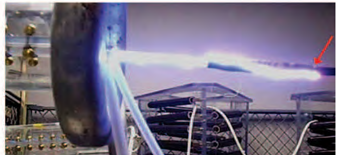
Figure 11. CUT#6. Photo of flashover. Positive polarity.
