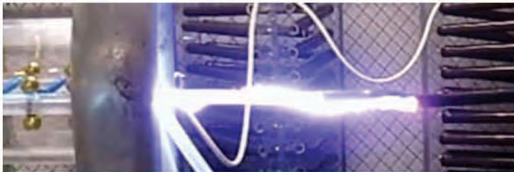
Figure 10. CUT#5. Photo of flashover. Positive polarity.
