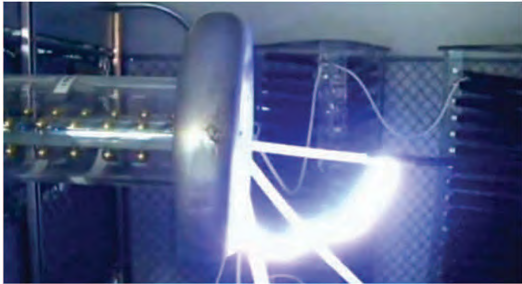
Figure 9. CUT#4. Photo of flashover. Positive polarity.
